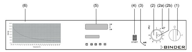
Figure 4: Control panel of FDL 115 standard unit
