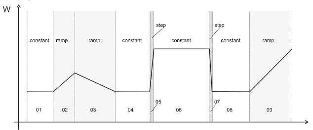
Figure 7: Possible temperature transitions (with default setting "Ramp" in the user level (chap. 10)
