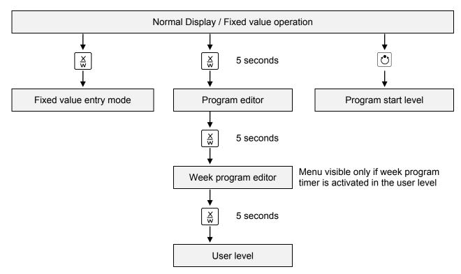
If no button is touched within more than 120 sec. the controller returns from the current level to Normal Display.
