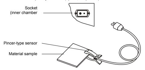
Figure 12: Sensor probes for optional temperature display
