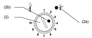
Figure 8: Safety thermostat class 2
