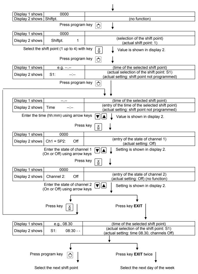
To exit the menu, press several times key **EXIT** or wait for 120 seconds. Controller returns to normal display.
